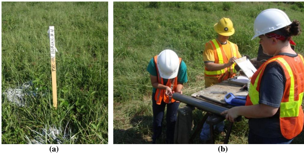
Figure 6.5. a) Pre-drilling conditions at B-4, and b) torvane test being performed in Shelby tube soil sample .
