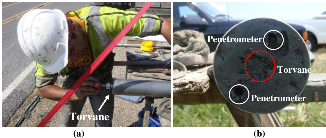
Figure 4.34. a) Torvane test being performed on a tube, b) index test locations.
