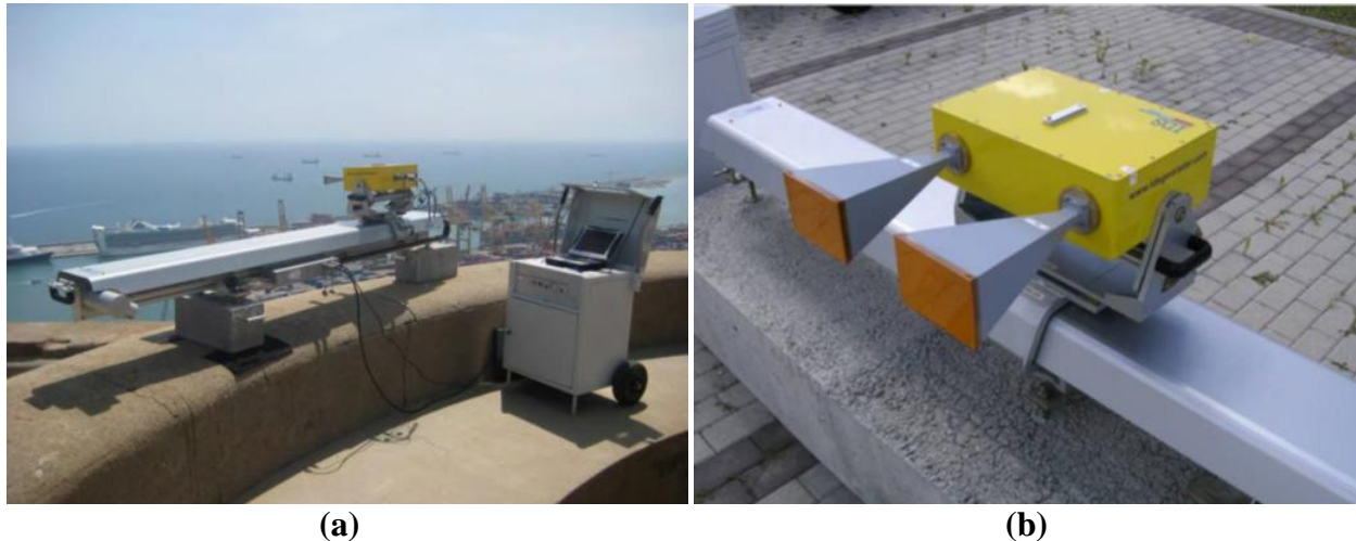
Figure 2.8.a) IBIS-L RADAR system: rail, sensor module, and computer/power component (from (Jungner, 2009), b) IBIS-L sensor module composed of receiver and transmitter antennas (from Ingegneria Dei Sistem Website, 2012)
