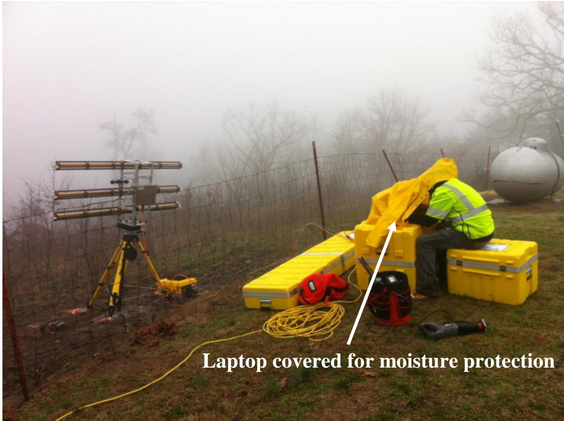
Figure 4.24. GPRI-II acquiring data during fog in overlook viewpoint (calibration site) near Chester, Arkansas.
