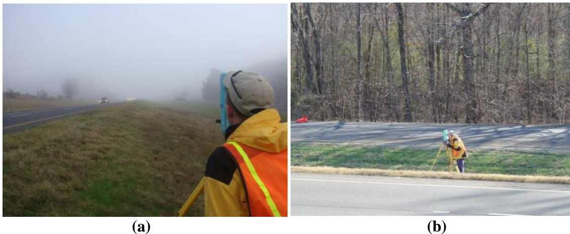
Figure 3.21.a) University personnel acquiring points for topographic model, b) looking South to the total station set up point in validation site near Malvern, Arkansas.
