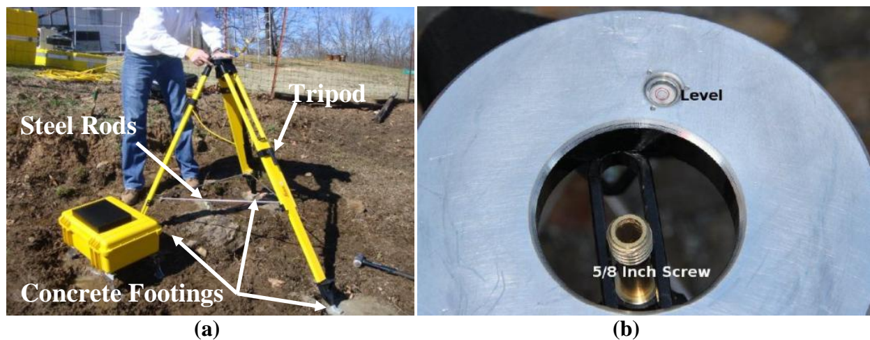
Figure 4.14. a) tripod for GPRI-II anchored to footings, b) tripod's bubble level (from GAMMA Remote Sensing AG, 2011).
