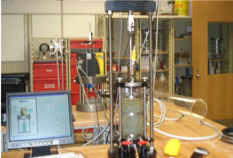
Figure 4.47. a) UU triaxial apparatus, and b) UU test being conducted in a soil specimen obtained from validation site near Malvern, Arkansas.
