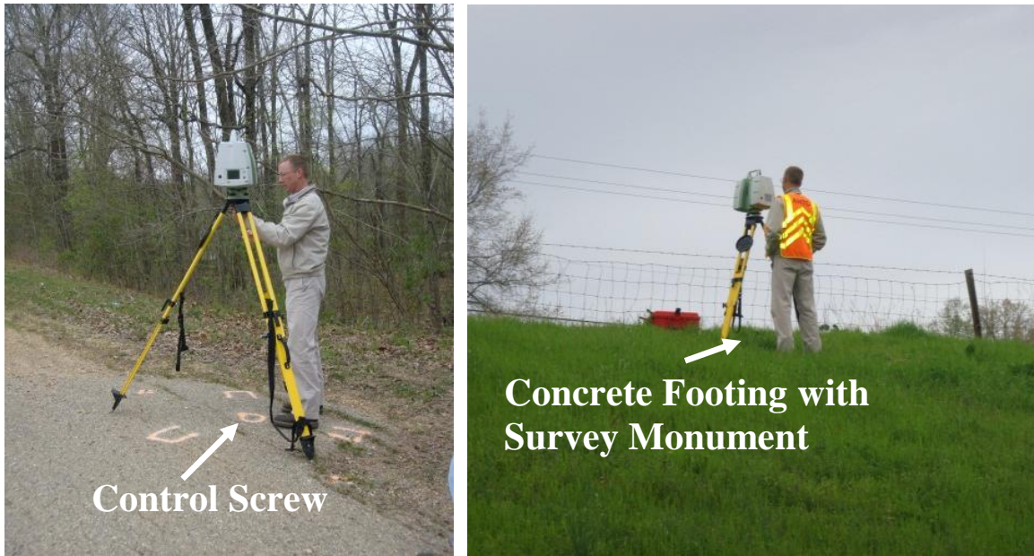
Figure 4.30. a) LIDAR being deployed at the NE viewpoint, and b) LIDAR acquiring data at the SW viewpoint.
